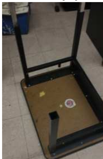
Loose and missing legs
